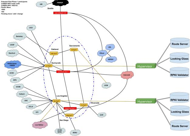
RPKI Validator instances synchronize their local ROA database with the (RIRs) trust anchors
