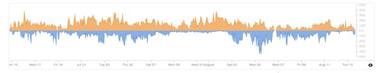
Observation: EU->US is only slightly higher than US->EU. Traffic direction is generally balanced on both LHCONE and LHCOPN.
